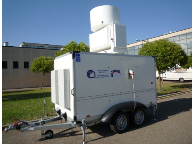
Figure 3.4: MIRA36 Ka-band Doppler radar operating at CIAO.
